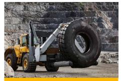
TYRE HANDLER The tool we have developed for a safe and gentle tyre change, reduces downtimes and damages.
